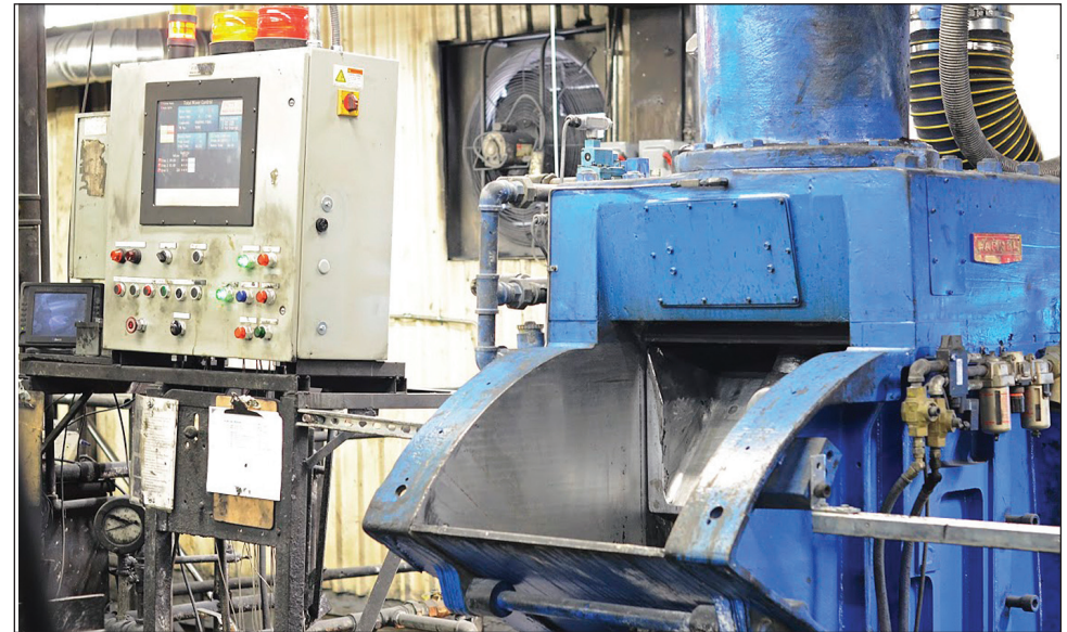
Polymeric's has put in a newly rebuilt No. 9 drop door mixing machine.
